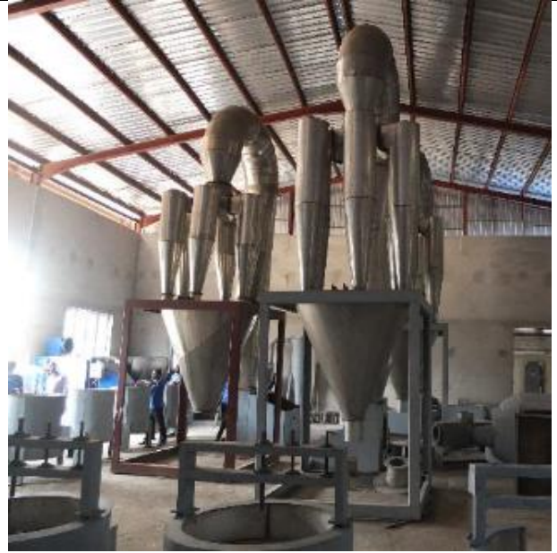
Production of 'six-cyclone' flash dryers at Nobex, Lagos
