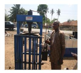
Materials Used: Mild steel (frame and hanger), stainless steel (press plate)
